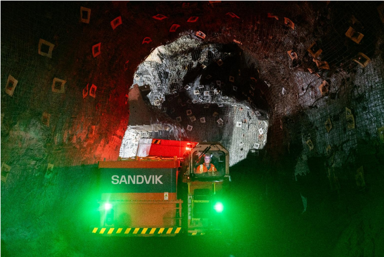
BEV Truck Loading on 150m level
