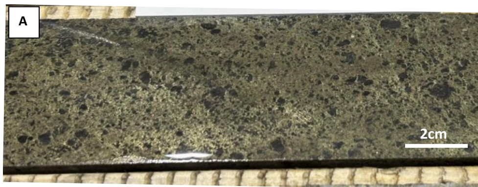
Figure 3. Photos of the McIlvenna Bay extension intersection in BZ-25-001, including A) chalcopyrite-rich massive sulphide equivalent to Lens 3 (1,231.0m depth); and B) sphalerite-rich sample within Lens 2 (Main Lens) mineralization (1,245.4m depth).
