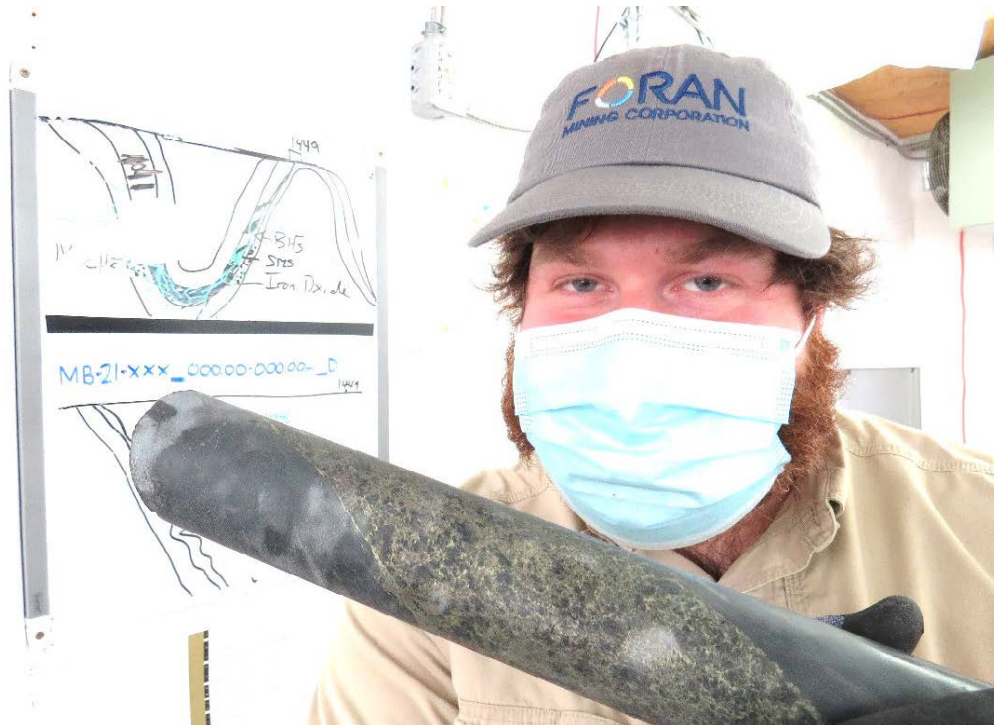
Geologist Sean Cross holding more splashy core...semi-massive chalcopyrite and pyrite in a sphalerite matrix.
